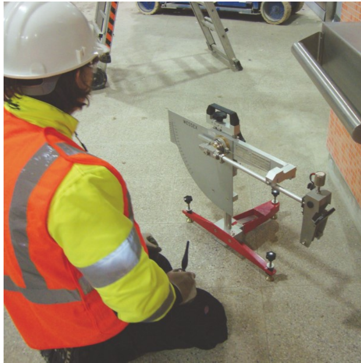
Figure 1: SATRA uses a machine with a swinging pendulum to measure floor surface resistance against BS 7976-2:2002+A1:2013
